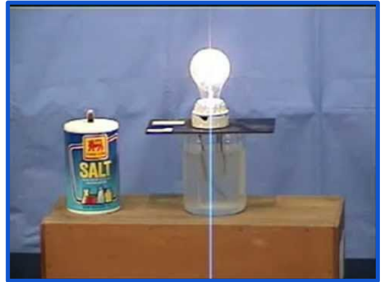
Example: Demonstration showing conductivity of salt water
